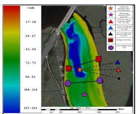
Figure 1: The dredge hole near Chestnut Neck is approximately 14-meters-deep. A vessel-mounted ADCP survey ran multiple transects over 6.5 hrs. within and adjacent to the hole. Supplemental data during the survey included three CTD casts (triangles) and a stationary ADCP within the hole (orange star). Velocity comparisons are made with previous survey data from a stationary ADCP downstream (pink star).
