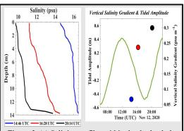
Figure 3: (a) Salinity profiles within the dredge hole on November 12<sup>th</sup> at three tidal stages (blue is early ebb; red is late ebb; black is slack tide) and (b) corresponding vertical salinity gradients (green line is water elevation). During ebb tide, the profiles show increased salinity at the bottom that persists as the tide changes and surface salinity decreases. This is confirmed by the increasing vertical salinity gradient.
